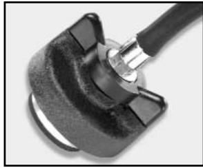
Tester head with pressure valve compressed.
